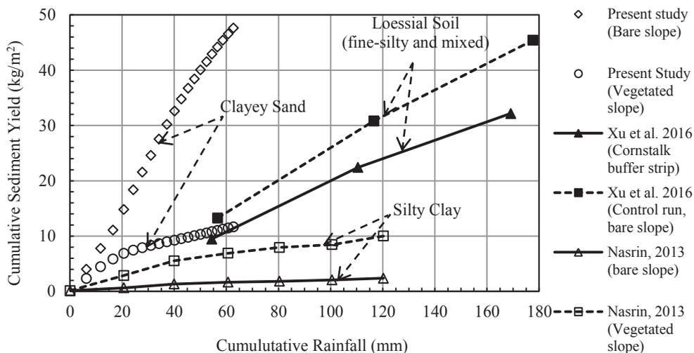
**Fig. 9.** Comparison of cumulative sediment yield due to rainfall for this study and experiment conducted by Xu et al. (2016) and Nasrin (2013) for bare and vegetated slope
