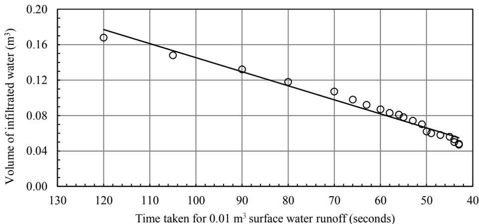
**Fig. 7.** Volume of infiltration vs. time taken for 0.01 m³ surface runoff
