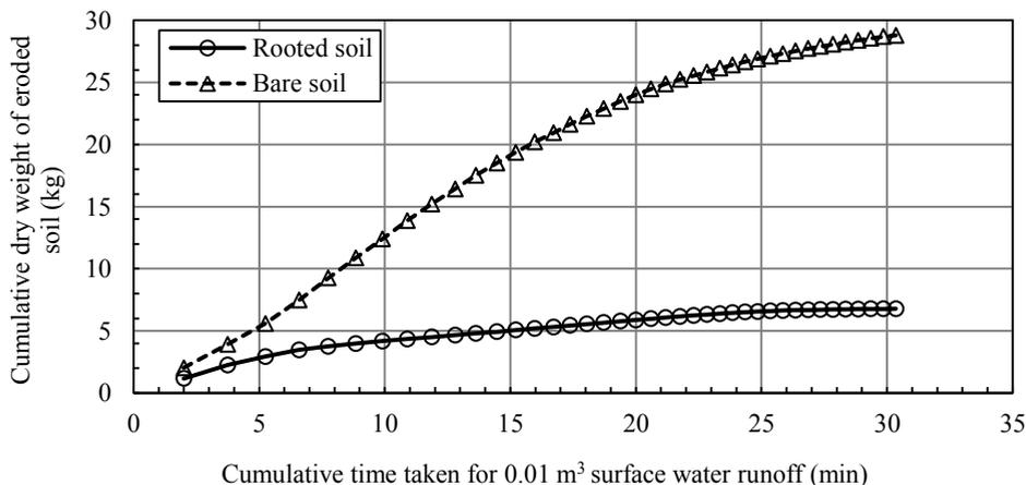
**Fig. 8.** Cumulative dry weight of eroded soil vs. cumulative time taken for every 0.01 m³ surface water runoff
